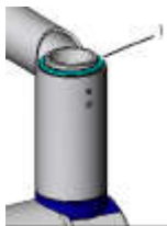
Fig. 37: Fit the locking ring
