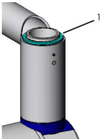
Fig. 24: Fit the locking ring
