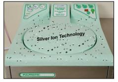
All DDC Dolphin macerators have the entire lid assembly impregnated with silver ion anti-microbial properties, reducing the risk of cross contamination. The cabinet is made from grade 304 stainless steel for easy cleaning, chemical resistance and high wear protection properties. This design offers more clinical safety and reduction in cross contamination.
