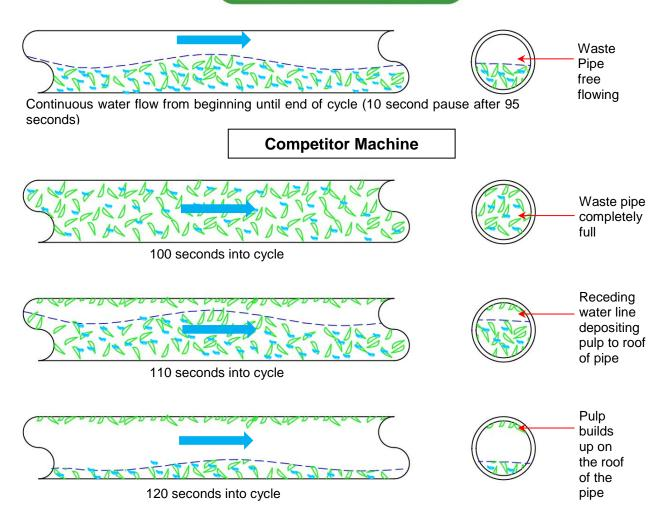
Blocked drains may also be the result of non-maceratable products being placed in the macerator, or a large amount of pulp trying to exit into the main drain over a very short release period. DDC Dolphin macerators combat both of these issues by keeping non-maceratable products within the upper chamber, and offering a steady flow of water and pulp which can only exit through the small 3.33 mm aperture, into drains.
