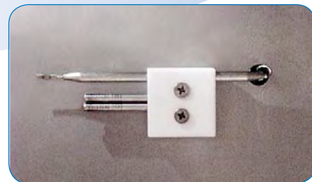
Hi-limit sensor (top), independent monitoring probe (middle), and control probe (bottom)
