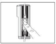
CAUTION: Ensure all four cassette latches are clearly visible after the cassette is installed. Refer to *Loading the Cassette* on page 35.
