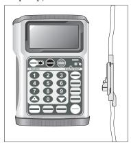
**4** Insert the cassette into the cassette pocket by pushing firmly along the entire cassette until it is firmly seated.
