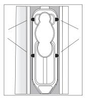
CAUTION: Ensure the cassette is properly installed. When properly installed, all four cassette latches are visibly holding the cassette securely in the cassette pocket.
