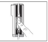
CAUTION: Ensure all four cassette latches are clearly visible after the cassette is installed. Refer to *Loading the Cassette* on page 35.
