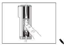
CAUTION: Ensure all four cassette latches are clearly visible after the cassette is installed. Refer to *Loading the Cassette* on page 35.
