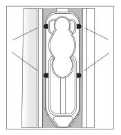
Note: Ensure the tubing is behind the tubing guide (at the distal end).
