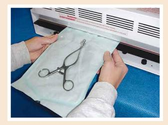
The Rennco Lift Seal™ Heat Sealer is easy to maintain as well as quick and simple to operate. Constant temperature is maintained by a digital temperature control during the sealing process. The lower silicone rubber bar is raised by a rugged mechanical drive to meet the stationary 1/2" wide heated sealing bar above. This bar is covered with a special "non-stick" fabric which is advanced by simply
