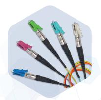
Belden's Fiber Express (FX) Fusion connectors enable splice-on technology. They combine the benefits of fusion splicing with the simplicity of a field-installable connector to expand your options for field-termination and improve installation performance and reliability over mechanical splice connectors. No crimping, polishing, or adhesives are required for termination, minimizing installation errors.
