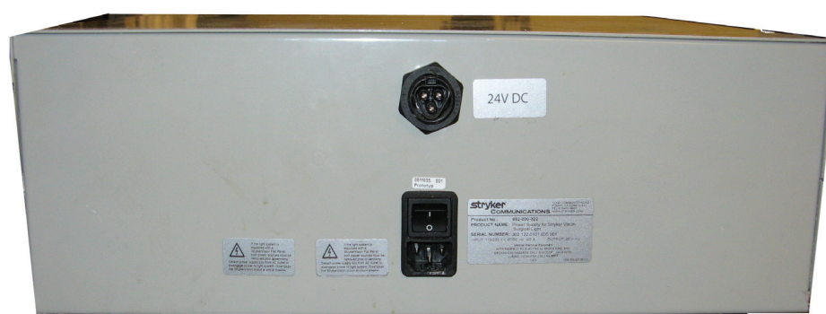
Back View of Power Supply Box
